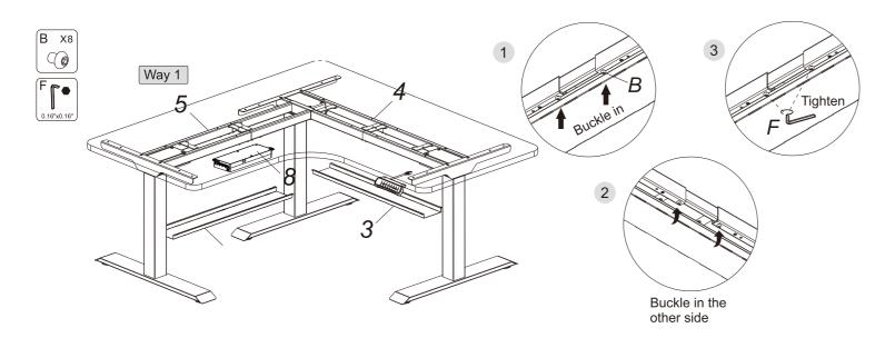
Firstly, screw the screw (B) into the supporting beam (4) with Allen Key (F), and not tighten completely. Buckle one side of the cable management tray (3) into the screw (B), then press the other side into the screw (B). Finally, the screw (B) is locked with Allen Key (F). The cable management tray (3) on the auxiliary beam (5) are installed in the same way.
