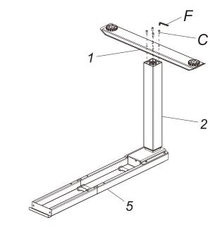
Install feet (1) and lifting column (2) together, use wrench (F) to tighten the screws (C).
