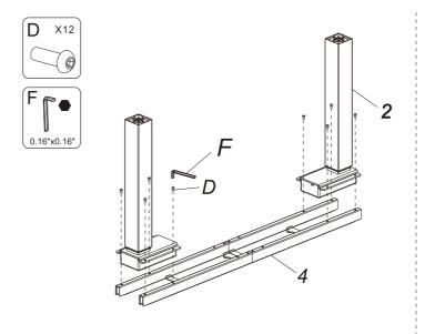
Install lifting column (2)and supporting beam (4) together, use wrench (F) to tighten the screws (D).
