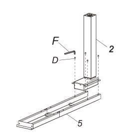
Install lifting column (2) and auxiliary beam (5) together, use wrench (F) to tighten the screws(D).
